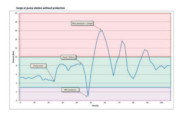
By installing a surge anticipator/pressure relief valve it is possible to reduce strongly the surge effects on the system.
