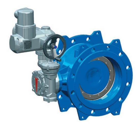
Double flanged double eccentric butterfly valve T.I.S. Type is designed to be installed in the pipeline in order to shut off the flow or limit it partially (indeed within certain limits double flange double eccentric butterfly valve could be also used as a control valve).
