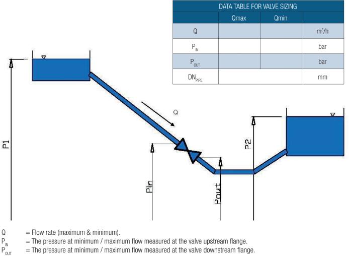
= The pressure at minimum / maximum flow measured at the valve downstream flange.
