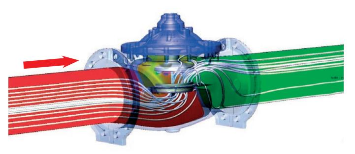
Automatic control valves, as defined by EN1074-5 standard: "have the integral capacity to control the function using energy from the conveyed water by adjusting the position of the shutter. They can be directly operated, i.e. the force is applied (via a spring or diaphragm) directly to the shutter." Alternatively, "They can be pilot operated i.e. the force is applied through an adjustable pilot valve".
