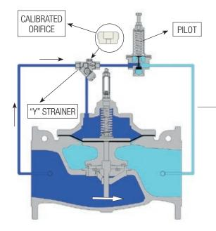
The pilot deviates upstream pressure into valve control chamber. The resulting pressure on the diaphragm moves the shutter to
