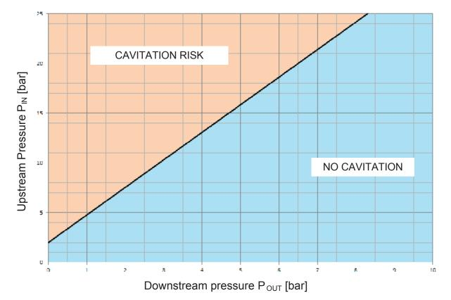
Cavitation diagram refers to 40% open valves. When the opening degrees of the valve significantly differs from this value, we recommend to verify the actual cavitation conditions by using the software specifically developed by T.I.S Nuoval. Please contact us providing valve's required operating conditions.
