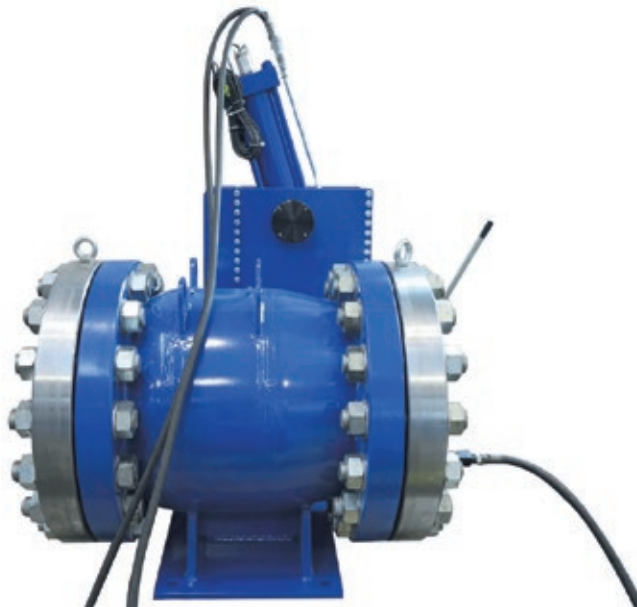
F600 PN100 HYDRAULIC TEST (PRESSURE TEST = 150 BAR)
